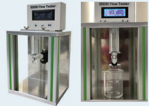
Bench-top design Dimensions: 200 × 150 × 345 mm Weight: 5 kg
