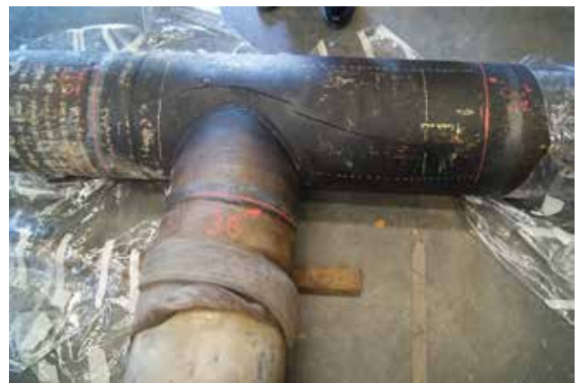
▲ Ruptured pipe sample for failure analysis
