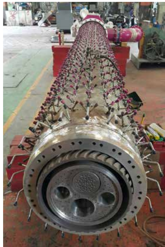
The kiln burner with anchors
