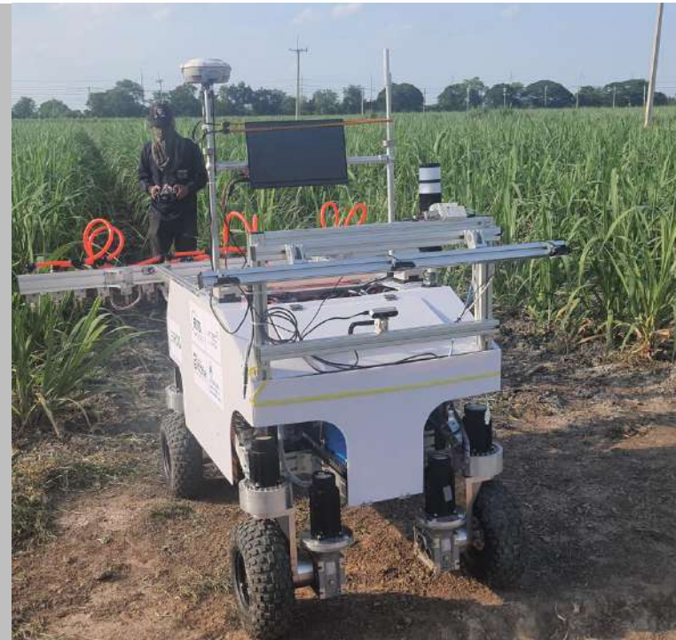
Terra: Automated agricultural mobile robot platform for weed control in sugarcane plantations
