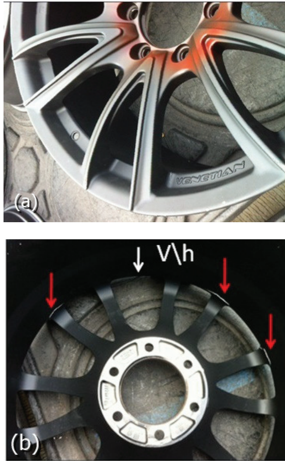
FIGURE 2. (a) Wheel geometry and (b) crack locations. In (b), all arrows mark the crack locations whilst the white one also indicates the valve hole (v/h) location.
